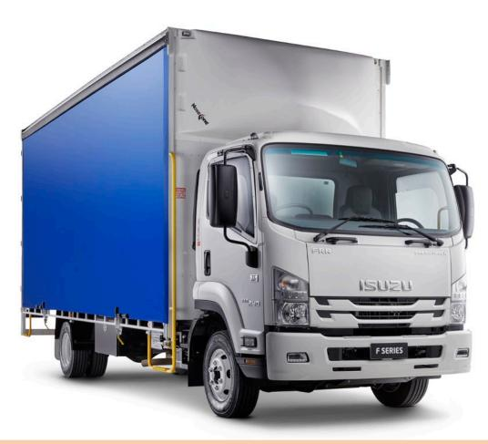
10 pallet (nominal) curtainside body / Easy glide curtains with quick release "Lightning" latches / Lightweight side gates / 3mm chequerplate floor and headboard with load restraints / Safety yellow coloured body steps and grab handles / Underbody mounted storage box / LED lighting for body interior and access steps / Body mounted air deflector / Body interior camera / Isuzu low light capable reversing camera / Daytime running lamps
